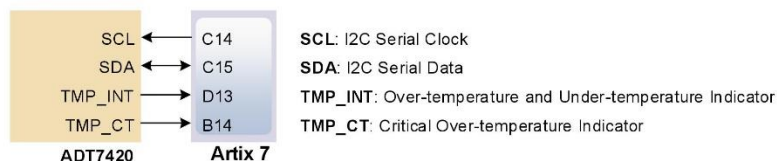
Figure 22. Temperature sensor interface.
